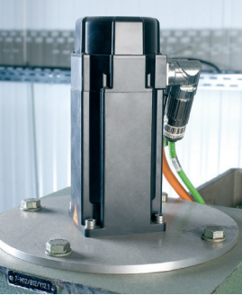
New Z-axis motor on the left. At the bottom: Position sensors are replaced when the original measuring device is damaged.
