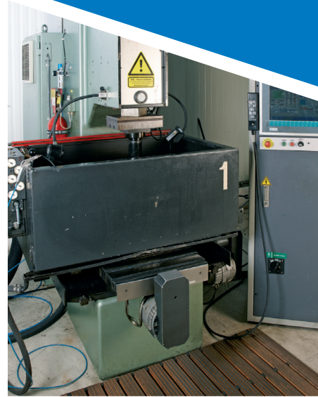
Using automatic level control also for the old machine. A new control system box on the right.
